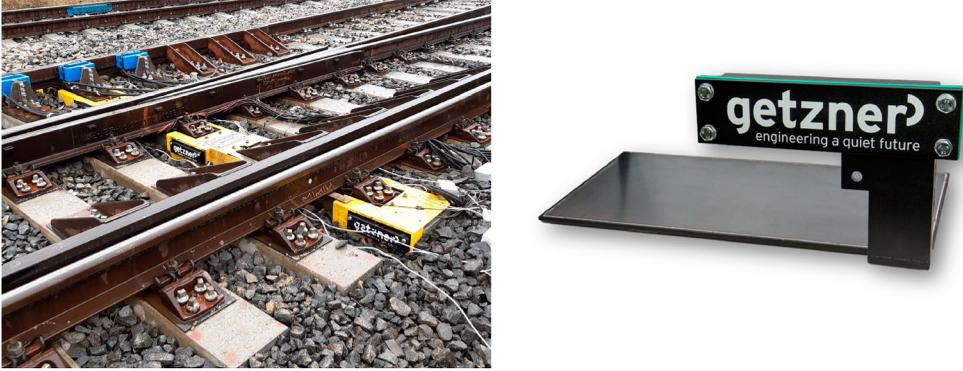
**Figure 3.** Sensor Sleeper in track (left) and individual sensor (right).
